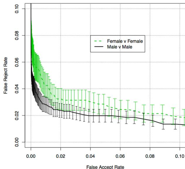
Figure 5: ROC curve corresponding to the fourth row of Table 3 for uncontrolled illumination and neutral expressions. Female vs. female (top green dashed line), male vs. male (bottom black solid line)
